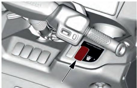
AUTOMATIC FIRE EXTINGUISHER INDICATOR LIGHT
