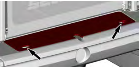
ANCHOR STORAGE COMPARTMENT COVER
