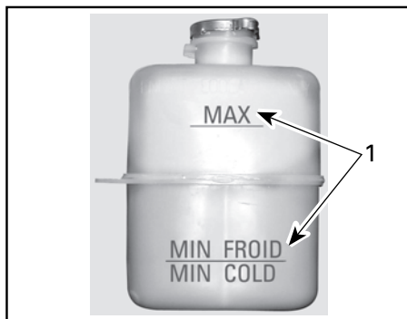
1. Level between marks when engine is cold
