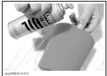
TYPICAL - OIL THE FOAM FILTER
