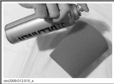
TYPICAL - SPRAY THE FOAM FILTER
