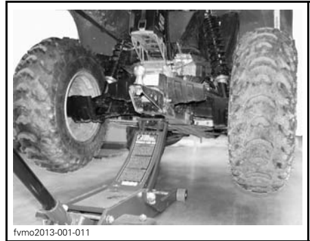
TYPICAL — BACK UP POINT LOCATION
