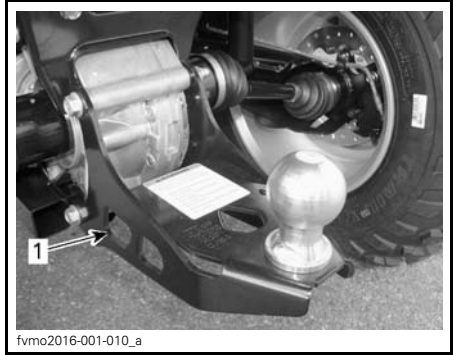
TYPICAL - REAR TIE-DOWN POINT LOCATION
