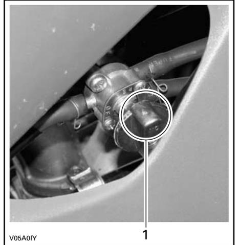
1. Align this pointer with the desired position
