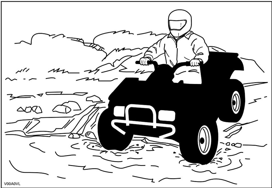
Water will affect the braking ability of your vehicle. Make sure you dry the brakes by applying them several times after the vehicle leaves the water.
