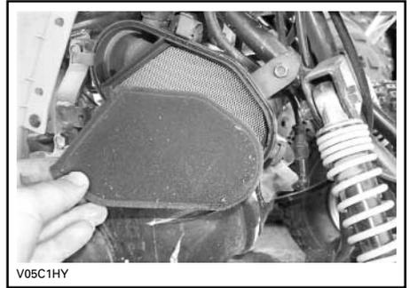
To clean the air filter element use the following procedure.
