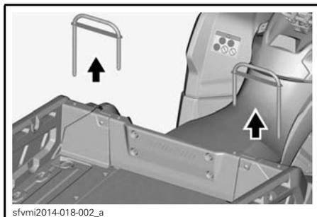
5. Lift side wall up and remove it.
