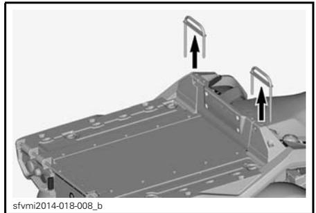
3. Place side wall on flat bed and lower it on its place.
