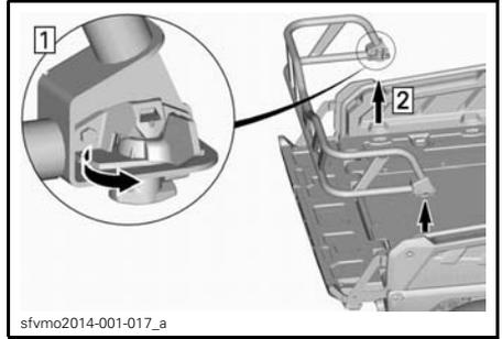
3. Remove support brackets from tail gate.
