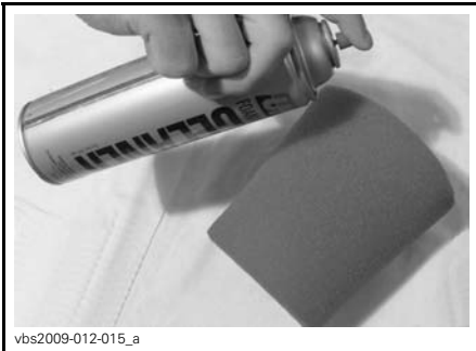
TYPICAL - SPRAY THE FOAM FILTER
