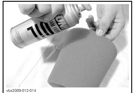
TYPICAL - OIL THE FOAM FILTER
