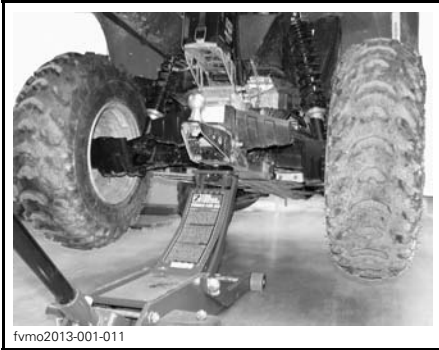
TYPICAL — REAR LIFTING POINT
