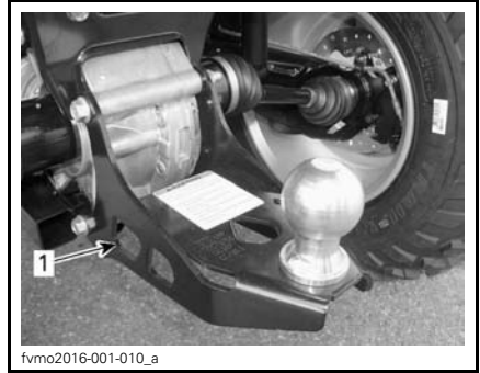
TYPICAL - REAR TIE-DOWN POINT LOCATION
