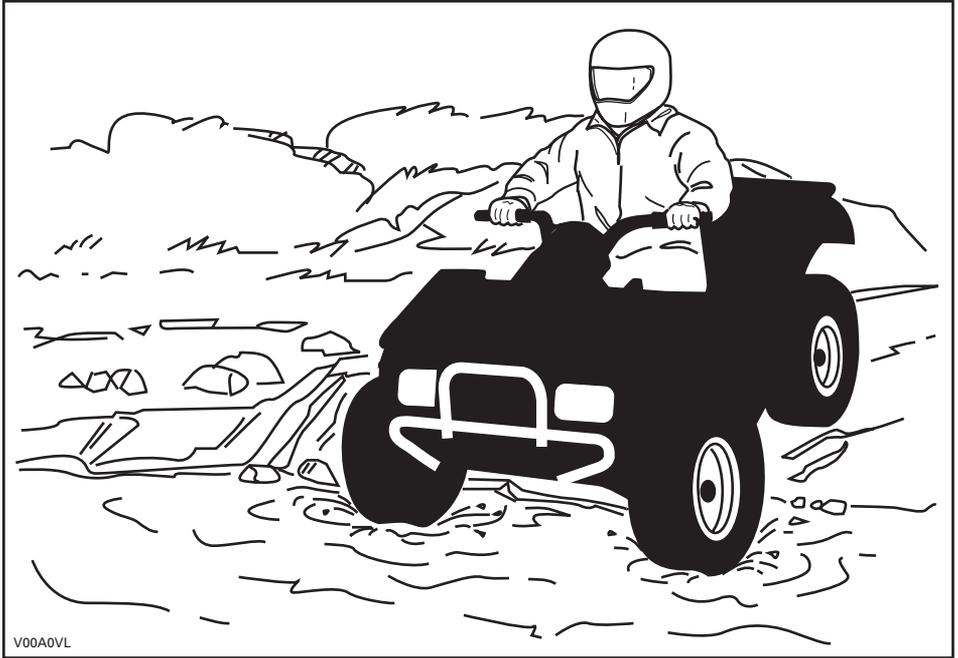
Water will affect the braking ability of your vehicle. Make sure you dry the brakes by applying them several times after the vehicle leaves the water.
