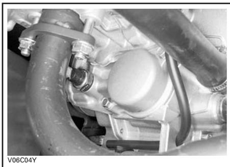
Remove oil filter and replace with a new filter.
