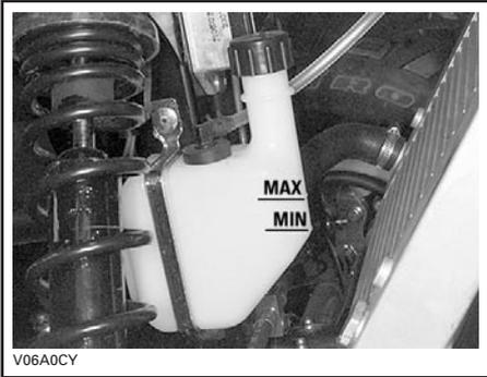
With vehicle on a level surface, liquid should be between MIN. and MAX. level marks of coolant reservoir.
