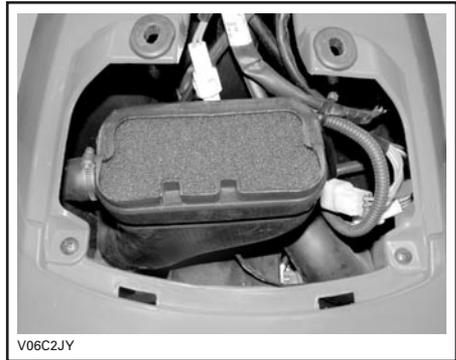
Pour cleaning solution (P/N 219 700 341) or an equivalent into a bucket. Put the filter in to soak.
