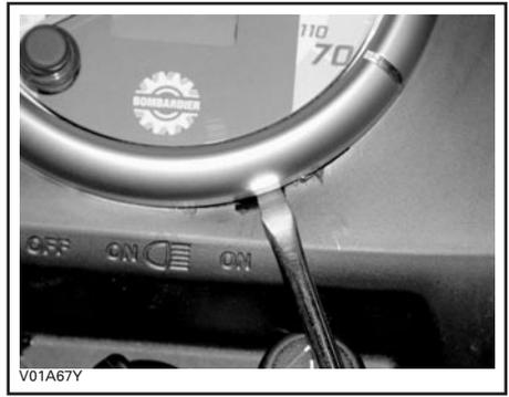
Unplug the auxiliary headlamp then turn the socket counterclockwise to unlock it. Pull the socket out of auxiliary headlamp housing and remove bulb.
