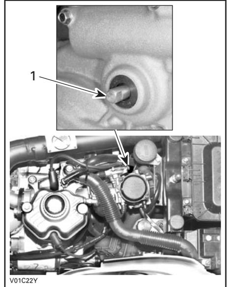
1. Emergency shifter shaft. Insert special tool here
