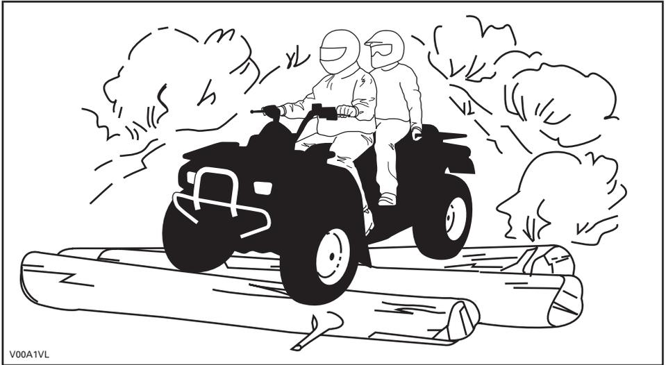
Even though there is an adequate suspensions system on this vehicle there are "washboard" or rough terrain conditions that will make you feel uncomfortable and even cause back injury. "Posting" or riding in a crouched position will often be required. Slow down and allow your flexed legs to absorb impact.
