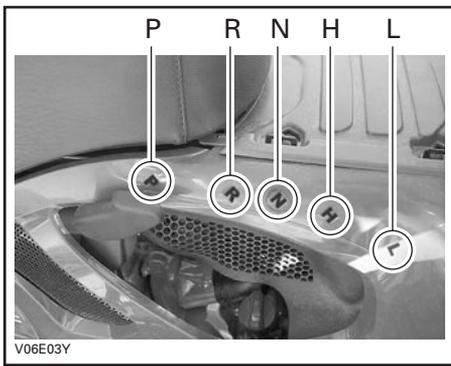
To change the transmission position, completely stop vehicle then move lever to the right then to the desired position while pulling lever upward. Do not force lever. If unable to shift, rock the vehicle back and forth to move the vehicle and try again.
