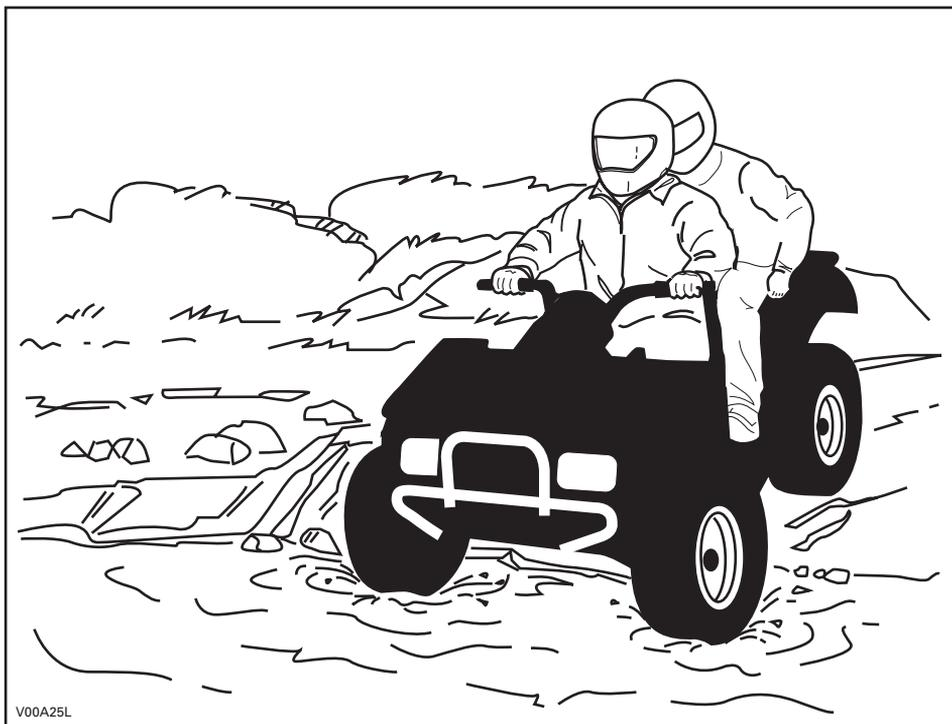
Water will affect the braking ability of your vehicle. Make sure you dry the brakes by applying them several times after the vehicle leaves the water. The vehicle braking distance may be affected when riding with a passenger. Safely reduce speed when riding with a passenger. Allow greater distance for braking.
