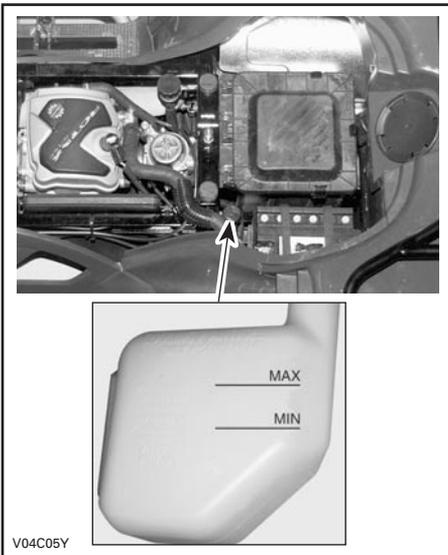
**NOTE:** When checking level at temperature lower than 20°C (68°F), it may be slightly lower than MIN. mark.
