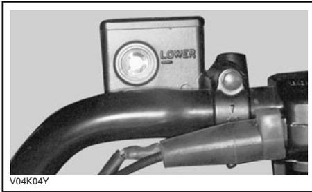
Visually inspect lever boot condition. Check for cracks, tears etc. Replace if damaged.
