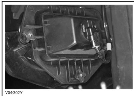
Rotate the bulb socket counterclockwise then remove headlamp.
