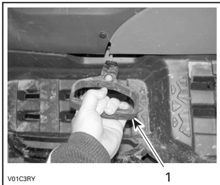
1. Grasp manual starter handle firmly and crank engine
