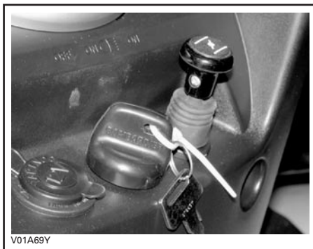
CHOKE KNOB LEVER IN THE OFF POSITION
