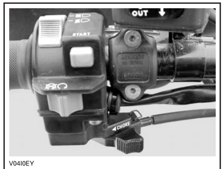
CHOKE LEVER IN THE OFF POSITION
