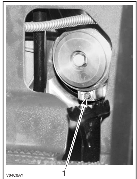
TRAXTER CVT — UNDER OIL FILTER COVER 1. Cooling drain plug
