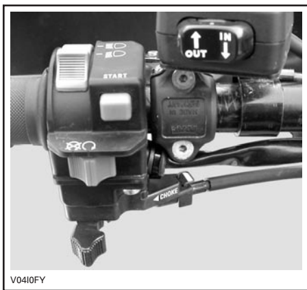
CHOKE LEVER IN THE FULL CHOKE POSITION
