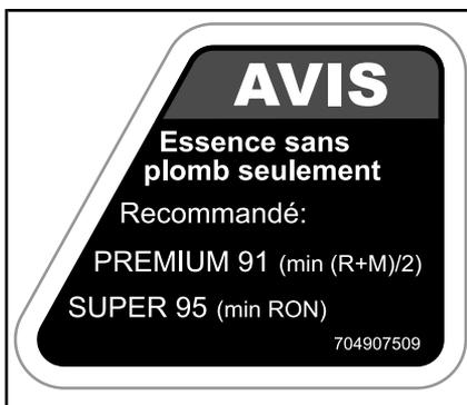
*À PROXIMITÉ DU BOUCHON DE RÉSERVOIR DE CARBURANT DU MOTEUR 1000R*
