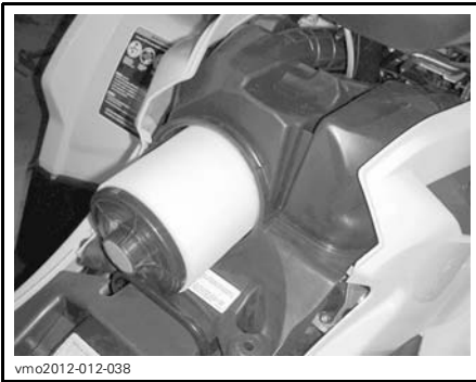
AIR FILTER REMOVAL
