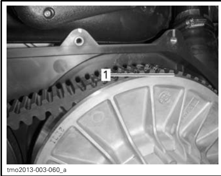
1. Lowest portion of cogs even with external surface of drive belt
