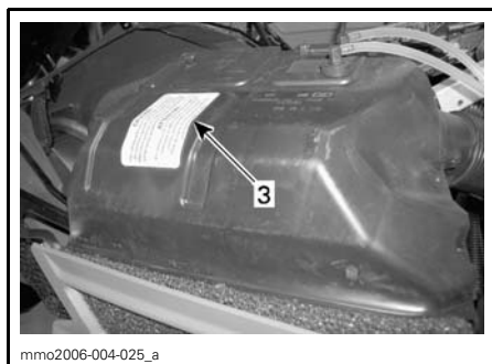
AIR INTAKE SILENCER (BODY SIDE) — FAN-COOLED
