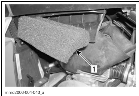
1. Removal of filter from its grill
