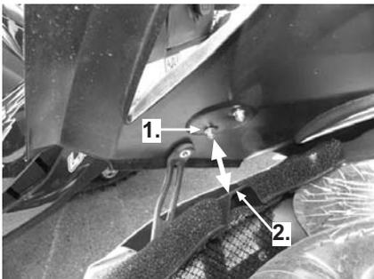
Install front of the hood then assemble rear part of hood to the openings.
