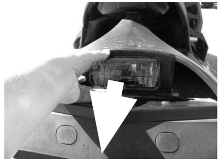
Turn bulb base to the counter clockwise to open the bulb base from tail light.
