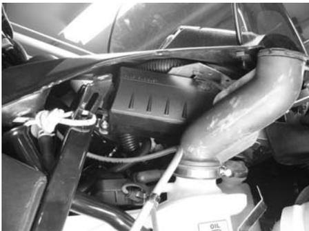
To open fuse box push on cover tab and tilt cover.
