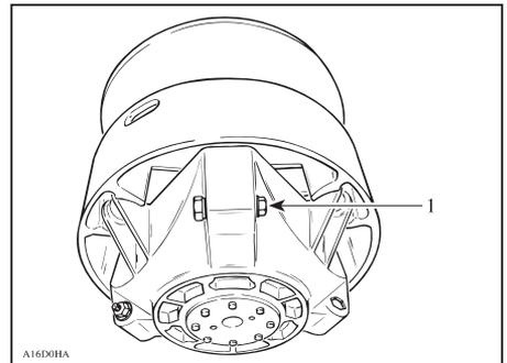
1. Loosen just enough to permit rotating of calibrate screw
