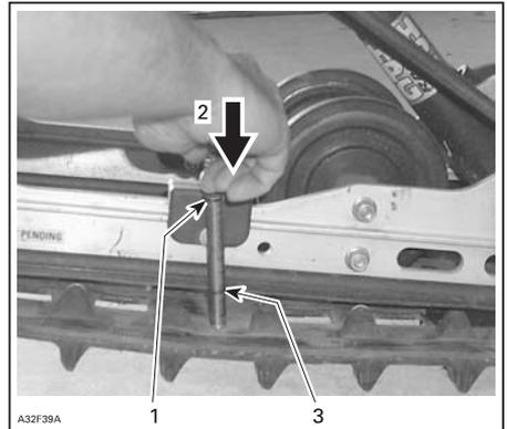
1. Top tool O-ring positioned at (example 7,3 kg, see technical data)
