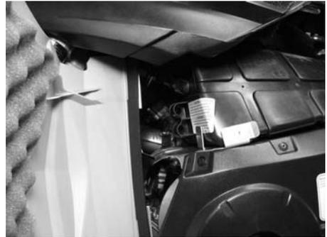
**Some models:** To keep spare spark plugs dry and prevent shocks that might affect the adjustment or break them, a holder is provided in engine compartment.
