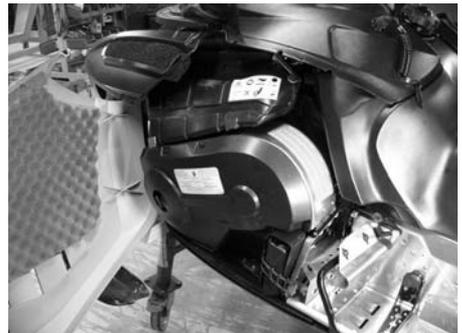
Lift up the intake silencer clamp.
