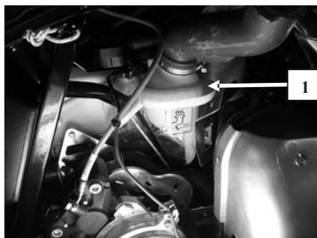
1. Max oil level. (Do not overfill)
