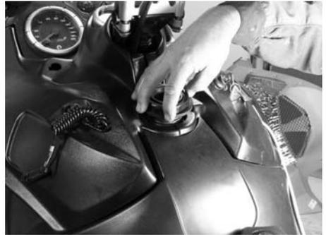
Lift console front edge up (pin in the rubber ring).
