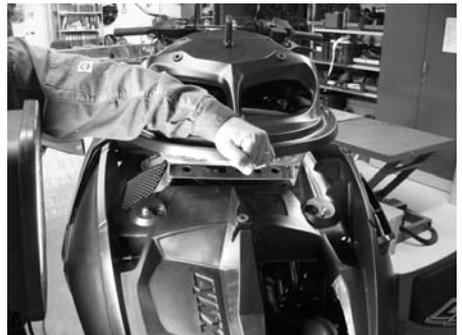
Lift the console rear edge until you have enough space to work with head lamp bulbs.
