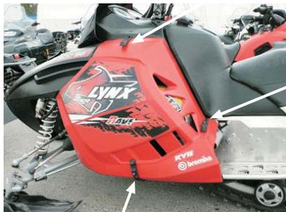
If you like to remove complete side panel, open the lockings and remove side hood.
