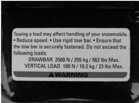
On this decal (in the picture), max. pulling load is 2500N vertical load for hitch is 10.2kg.
