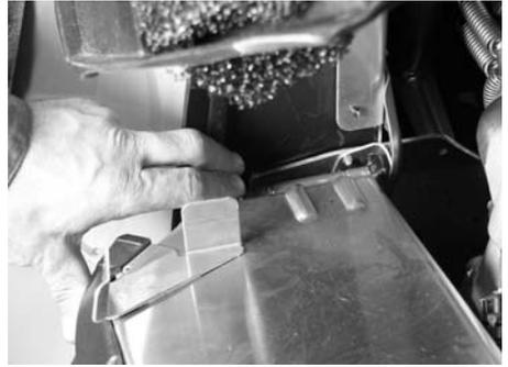
Lift cover front side up and bend it to out from unit to get it removed.
