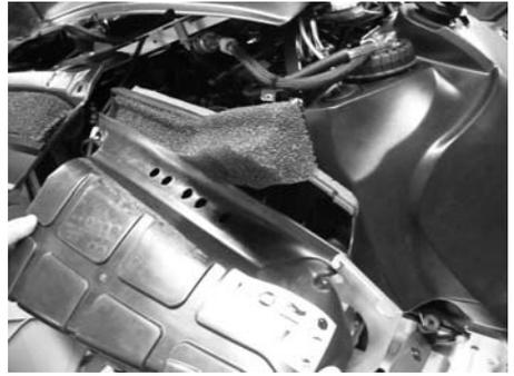
Check that the air silencer is clean and dry and properly reinstall the filter.
