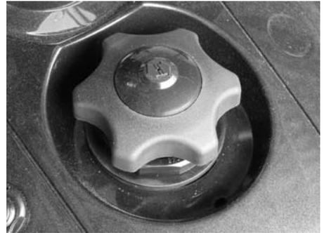
Unscrew to fill up tank then fully tighten.
