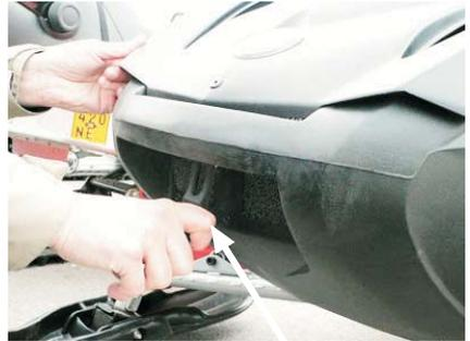
Open electrical connector at right side of vehicle by pressing the connector locking before lift up upper hood.
