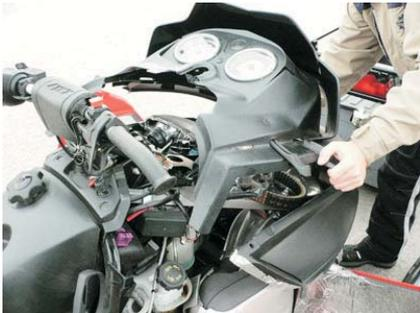
When assemble upper hood install nut [1] to the hole [2] on the bottom pan and fix the front latch to its position.
