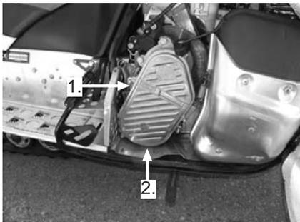
Set barrel below the chaincase and open the drainplug [2] and let the oil run out to the barrel.
