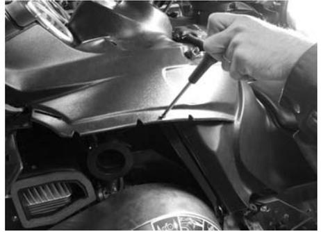
Open console big plastic nut round the fuel tank refill hole.
