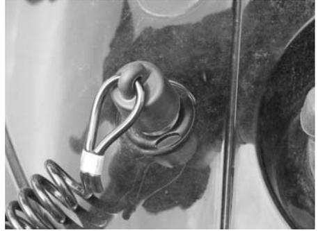
It shuts off engine preventing snowmobile to runaway if the operator falls off the vehicle accidentally.
