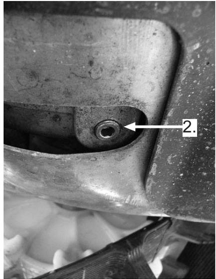
When oil is out from chaincase, close the drainplug.
