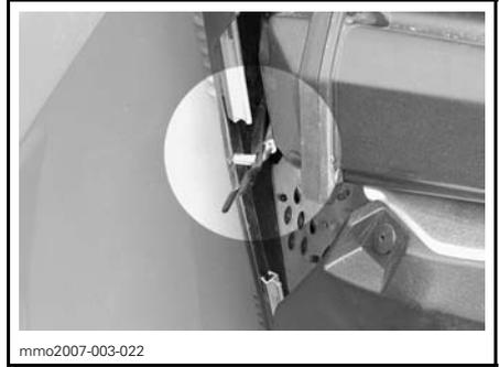
**FRONT RETAINING PIN PROPERLY SECURED**
