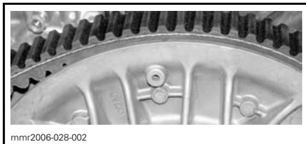
– Loosen both driven pulley adjusting nuts.
