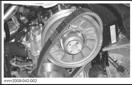
When drive belt is in position, driven pulley sheaves needs to be adjusted to obtain proper drive belt adjustment.
