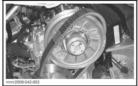
Remove drive belt from drive pulley.
