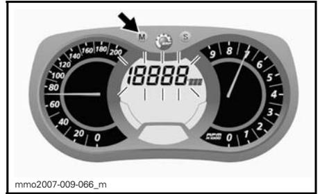
Push and hold the SET (S) button with in 5 seconds.
