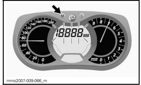
Push and hold the SET (S) button within 5 seconds to reset.
