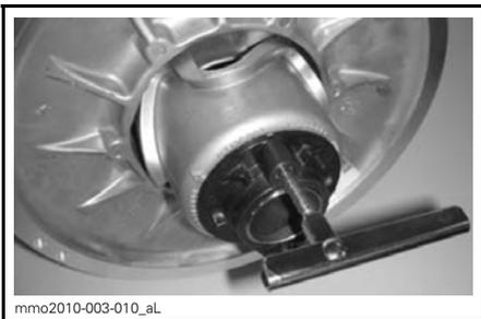
5. Open the driven pulley by screwing the tool in.
