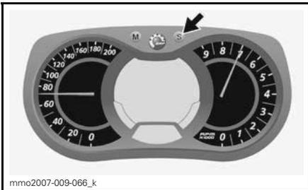
To change HOURS, while the value of HOURS is blinking, use the SET (S) button to change hours.
