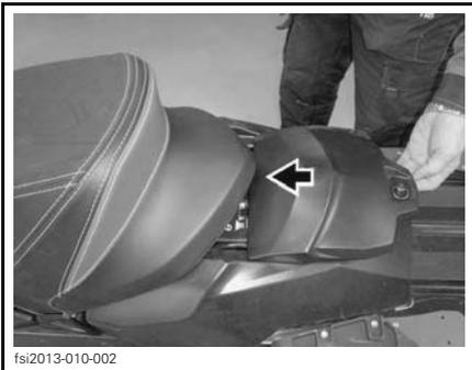
Finish the installation by locking the storage / battery compartment cover.
