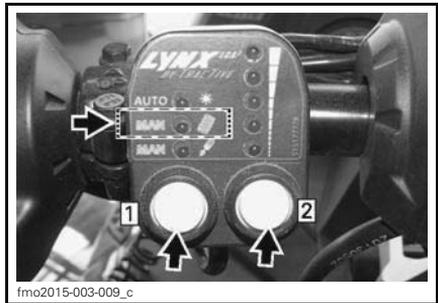
To adjust spring preload push the left button till the MAN/spring figure led lights up. Push the right knob to set the preload. Upwards is more preload and down is less preload.
