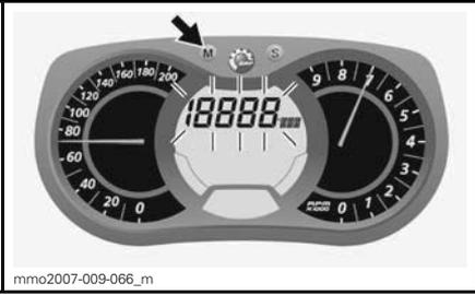
While display flashes, press and hold the SET (S) button within 5 seconds to reset.
