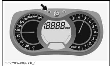
To reset, set the trip meter to TRIP B. Refer to *TRIP METER A OR B* for more details.
