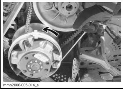
Pull the rope using a sharp, crisp pull so the rope comes free of the drive pulley. Start engine as per usual manual starting.
