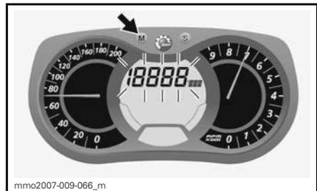
While display is flashing, press the SET (S) button to select altitude mode.
