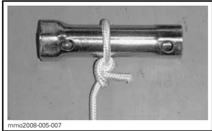
Attach the other end of emergency rope to the starter clip supplied in the tool kit.
