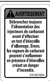
*SUR LES INJECTEURS DE CARBURANT - MODÈLES E-TEC*
