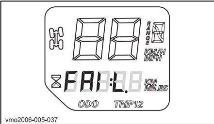
If your speedometer shows FAIL in the multi-function display, it means that the speedometer as sensed 18 volts in the electrical system, caused by a disconnected or defective voltage regulator.
