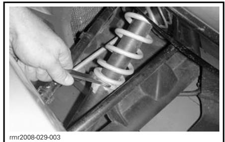
FRONT SUSPENSION CAM ADJUSTMENT
