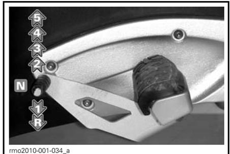
Lift up or press down fully to move sequentially from one gear to the next. When the lever is released, it returns to center where the mechanism resets for the next shift up or down. Neutral (N) is selected by either a half lift from first gear or a half press from second gear. Refer to *8) SHIFTING (p. 67)* for detailed instructions.
