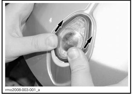
2. Lift front portion of lens with your thumb or a small screwdriver to release.
