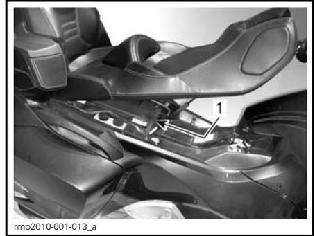
1. Fuse box located under the seat
