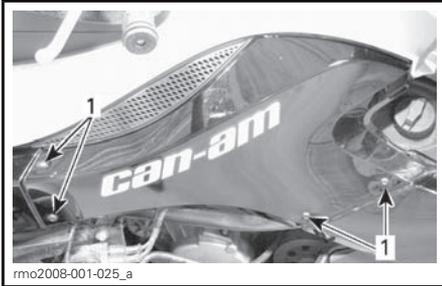
1. Parafusos Torx do painel lateral superior
