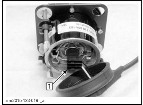
Step 1: Remove connector from light bulb
