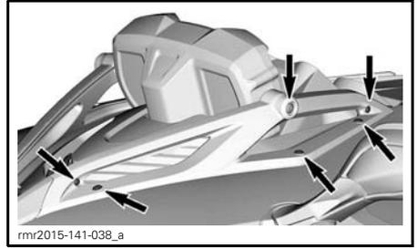
TYPICAL - RETAINING SCREWS TO REMOVE
