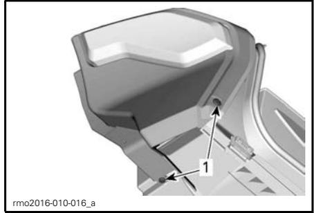
1. Lower retaining screws to remove
