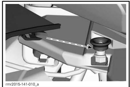
**TYPICAL - ALIGNING TABS IN CORRECT INSTALLATION LOCATION**
