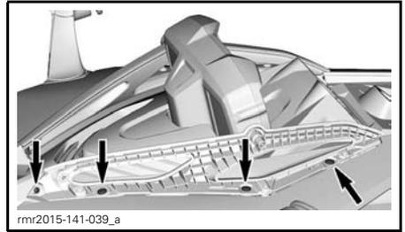
TYPICAL - RETAINING SCREWS TO REMOVE
