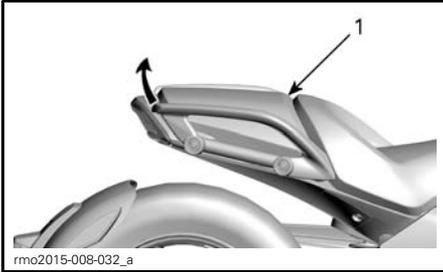
**TYPICAL - LIFTING PASSENGER SEAT TO REMOVE IT**
