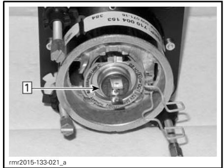
Step 1: Pull bulb out of light housing
