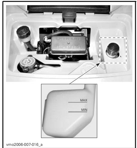
With vehicle on a level surface, liquid should be between MIN. and MAX. level marks of coolant reservoir.
