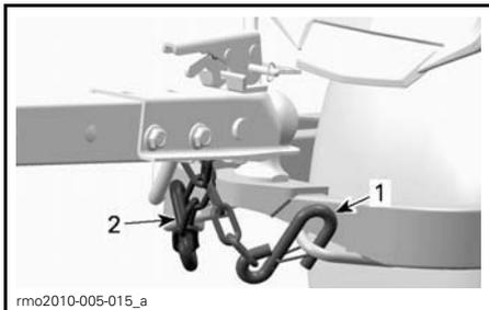
1. Left safety chain attaches on right side of hitch
