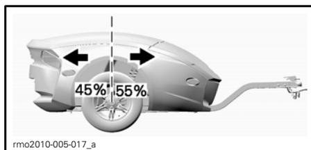
For partial load, place cargo at front. If the maximum tongue weight is reached, distribute remaining cargo toward rear.
