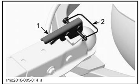
1. Coupler-locking mechanism in locked position
