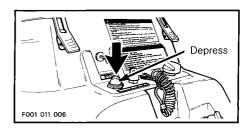
NOTE: Do not depress the throttle lever while starting a cold engine.
