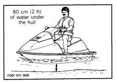
CAUTION: The engine must be stopped before less than 60 cm (2 ft) of water be underneath the hull. Otherwise shells, sand, pebbles or other objects could be drawn up by the jet pump and damage impeller, components or clog cooling system as well as jamming.
