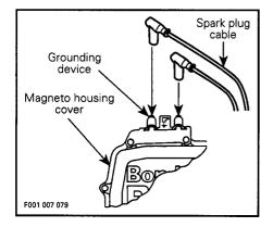
Remove both spark plugs and spray some SEA-DOO LUBE into each cylinder.
