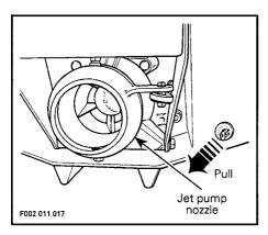
Tilt the watercraft slightly to the rear so that the water can completely flow out of the bilge.
