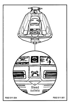
When engine is running, water must flow from these holes. This allows air in tuned pipe and in engine water jacket to escape. It also indicates that water is circulating in the cooling system.
