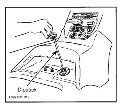
The dipstick indicates the amount of oil to be added in the reservoir. Oil level should be maintained between FULL and ADD marks. Before checking oil level, place the watercraft level, then wipe the dipstick and insert it in the reservoir neck. Do not screw cap. Remove dipstick and read the level.
