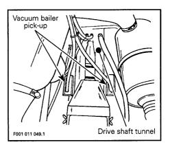
This watercraft features a vacuum activated syphon. Two bailer pick-ups use a low pressure area in the jet pump to syphon the water out of the bilge.
