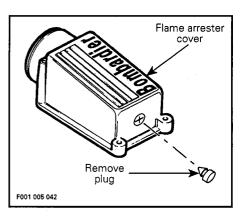
Spray some SEA-DOO LUBE (P/N 293 600 006) through flame arrester cover keeping engine at fast idle. CAUTION: Do not use outboard type storage lubricant. Using outboard lubricant may accelerate corrosion and damage engine components.
