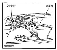
Visually inspect the oil filter at least every 10 hours. Ensure that it is free of water, clean and no foreign particles are present, if so, refer to an authorized dealer for replacement.
