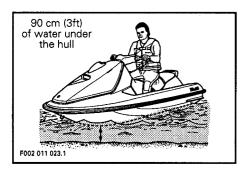
CAUTION: The engine must be shut off before less than 90 cm (3 ft) of water is underneath the hull. Shells, sand, pebbles or other objects could be drawn up by the jet pump and damage impeller, components or clog or jam cooling system.
