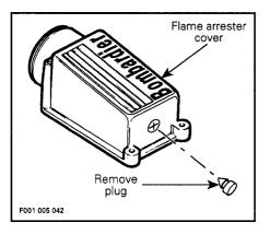
Spray some SEA-DOO LUBE (P / N 293 600 006) through flame arrester cover keeping engine at fast idle.
