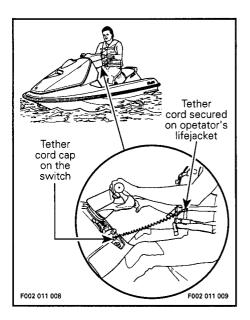
WARNING: Should the engine be stopped, watercraft directional control is not available.
