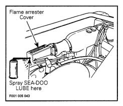
Lubrication of engine should be done at least for one minute. After approximately half a minute, close fuel tank valve to run engine out of fuel while lubricating.
