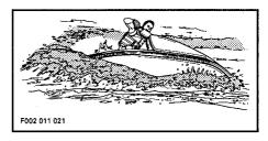
Turning the handlebar pivots the jet pump nozzle which controls the watercraft direction. Turning the handlebar to the right will turn the watercraft to the right and inversely. The throttle must be applied to turn the watercraft.
