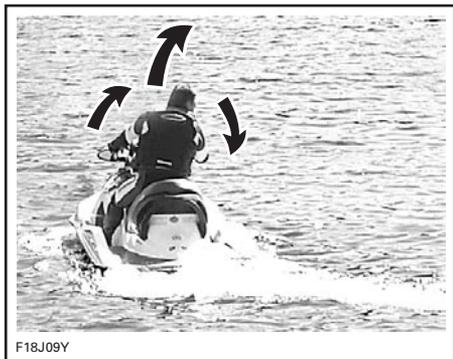
Turning the handlebar pivots the jet pump nozzle which controls the watercraft direction. Turning the handlebar to the right will turn the watercraft to the right and inversely. The throttle should be applied to turn the watercraft.
