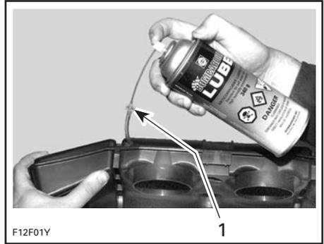
1. Partially pull tube out of air box to inject BOMBARDIER LUBE lubricant or equivalent. Push tube in when finished
