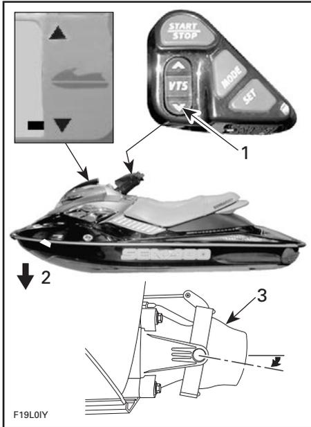
1. Push on arrow pointing downward on VTS button
