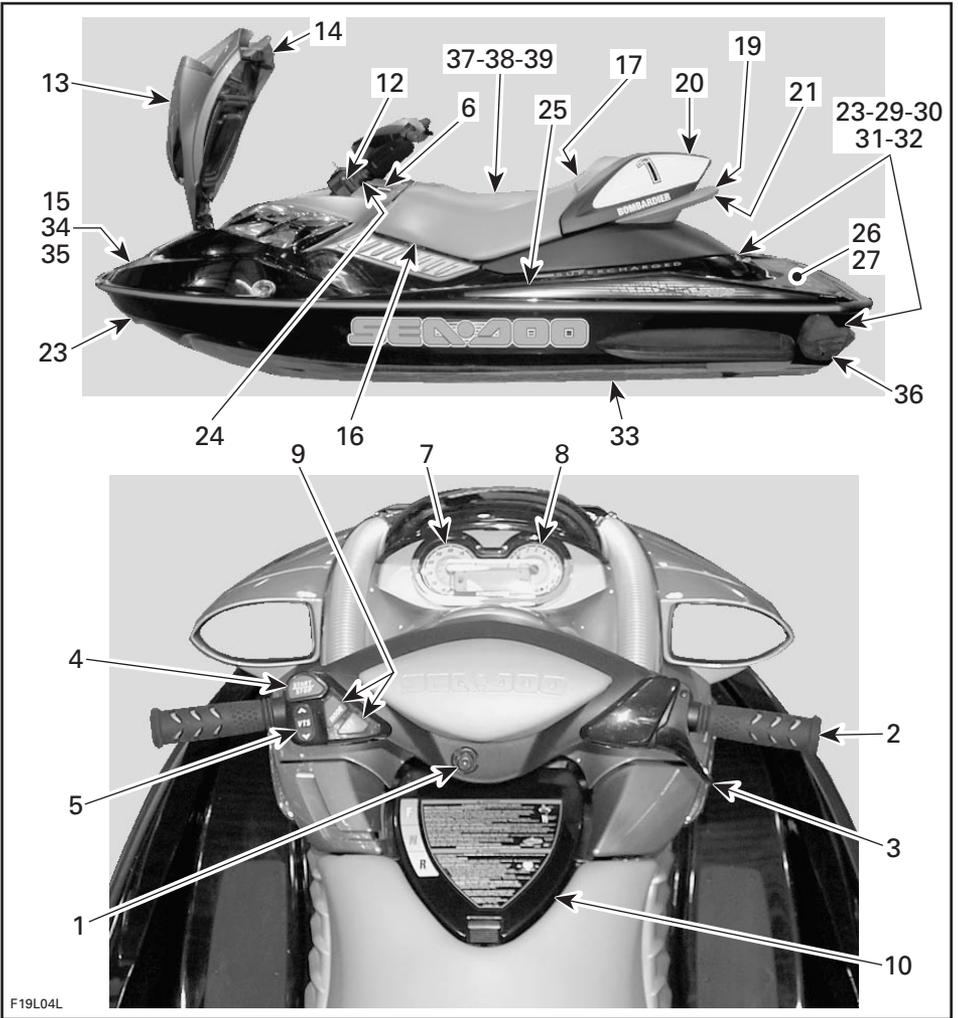
1. Safety Lanyard (engine cut-off cord)
