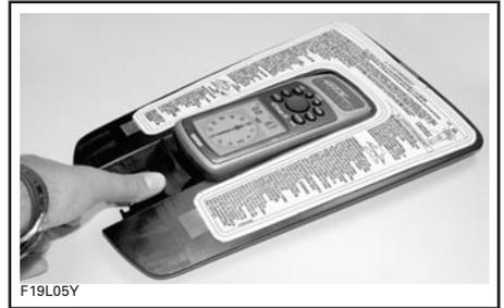
To reinstall, position GPS receiver in its receptacle and push until it latches.
