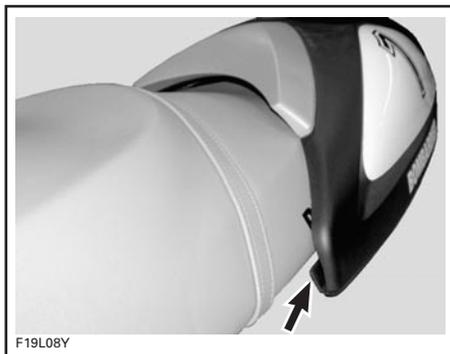
Finish pushing cover in position then lock the quarter-turn screws.
