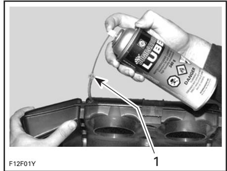
1. Partially pull tube out of air box to inject XP-S Lube lubricant or equivalent. Push tube in when finished.
