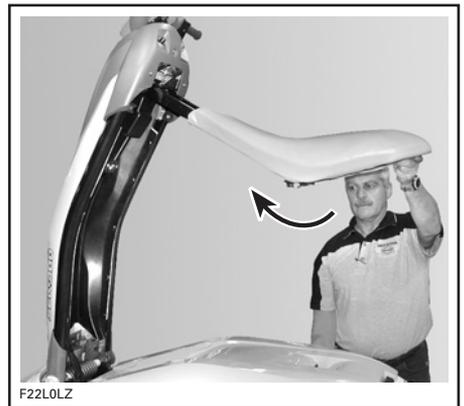
**CAUTION:** Make sure to maintain the steering pole high enough so that the “moto” seat clears the engine cover when rotated forward into the pole.
