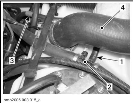
1. Disconnect the water supply hose (identified with a red tape)
