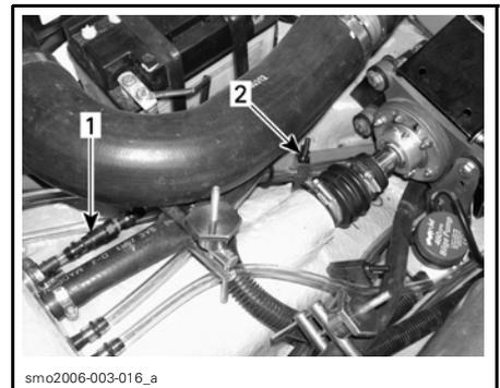
1. Engine magneto drain hose
