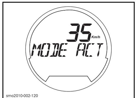
**MESSAGGIO SCORREVOLE - SKI MODE ACTIVE - PRESS\_MODE\_AND RETURN TO IDLE TO CANCEL (MODALITÀ SKI ATTIVA - PREMERE MODALITÀ E TORNARE ALLA VELOCITÀ DI MINIMO PER ELIMINARE)**
