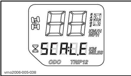
If your speedometer shows **SCALE** in the multi-function display, it means that the display selector button is stuck in the down position or depressed when the electrical system was activated.
