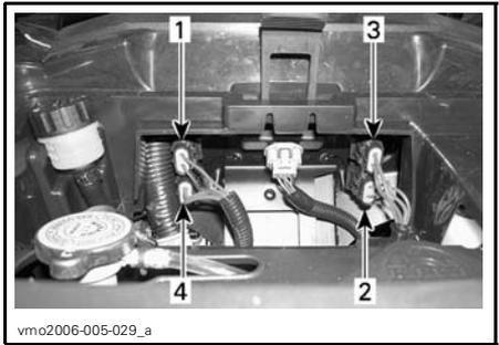
1. Accessories (15 A) (power outlet and auxiliary supply)
