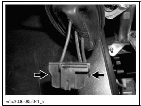
**PUSH ON LOCKING TAB TO UNLOCK CONNECTOR**
