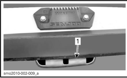
1. Hooked portion of rack in lower bracket
