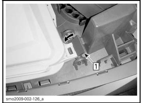
Step 1: Push down onto latches to secure
