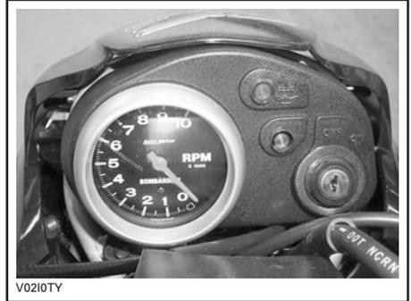
The tachometer indicates the revolution per minute (RPM) of the engine. Multiply by 1000 to obtain an approximation of the actual RPM.
