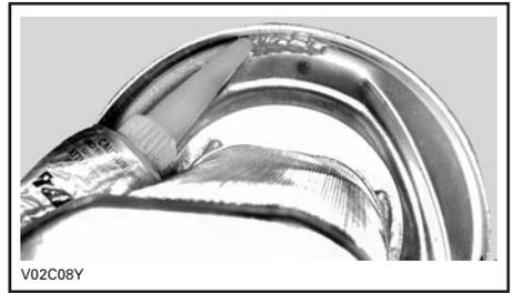
Be sure that wool is in place when inserting grill.
