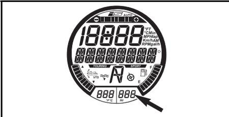
DISPLAY DO MEDIDOR DE HORAS
