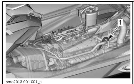
1. Tuyau de raccordement
