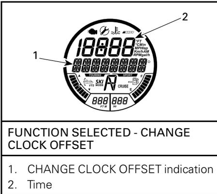
4. Press the UP/DOWN button to adjust the clock to the correct local time.
