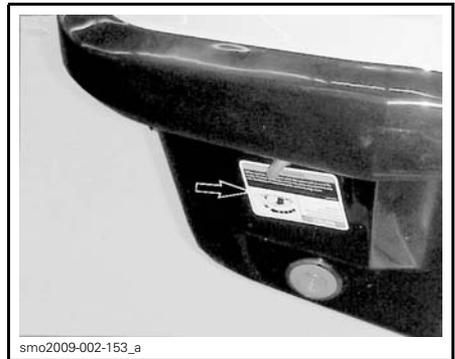
The 4-TEC™ engine features a tip-over protection system (T.O.P.S.™). When the watercraft tips over, the engine is automatically stopped.
