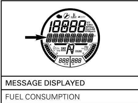
2. Press the UP/DOWN button to toggle to the desired fuel consumption display mode.
