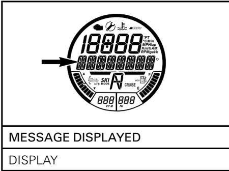
2. Press the SET button to enter the DISPLAY function.
