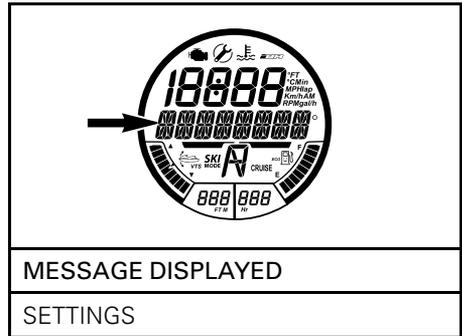
2. Press the UP/DOWN button repeatedly until CLOCK is visible.
