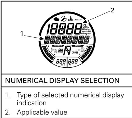
4. Press the SET button to select and save the preferred indication, or wait for the display function to time out. The last indication visible will be automatically saved.
