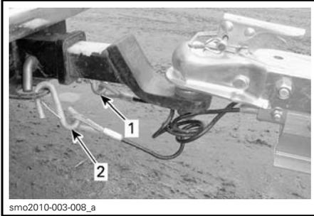
1. LH tongue safety cable attached to the RH side of hitch
