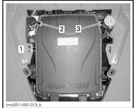
1. Engine air filter housing cover
