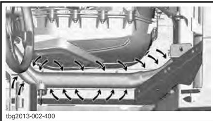
2. Using a garden hose, thoroughly clean the area so that no more debris can be in contact with the exhaust.
