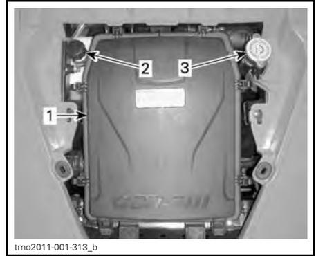
1. Engine air filter housing cover
