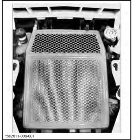
3. Verify that the cover fits well on the engine air filter housing before closing clamps.
