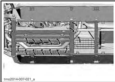
2. Using a garden hose, thoroughly clean the area so that no more debris can be in contact with the exhaust.
