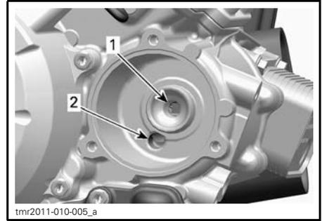
1. Outlet to the engine oil providing system
