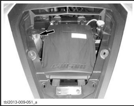
Coolant should be at the **MIN** mark when engine is **COLD**.
