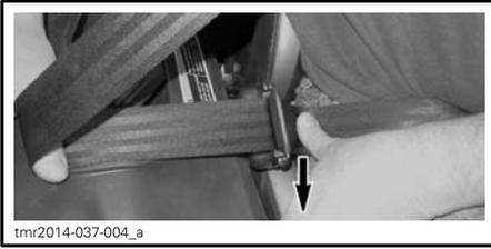
To release the seat belt, push on the red button on the seat belt buckle.
