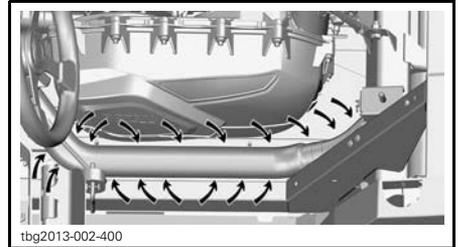
2. Using a garden hose, thoroughly clean the area so that no more debris can be in contact with the exhaust.
