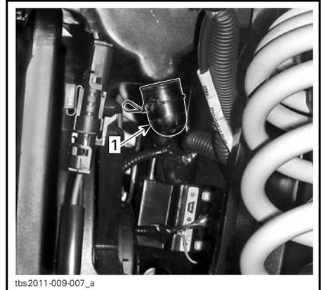
**ACCÈS AU BOUCHON DE VIDANGE DU CÔTÉ GAUCHE DU VÉHICULE**
