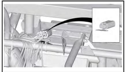
DRITTER SICHERUNGSKASTEN - HINTER OBERER KONSOLE
