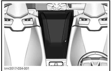
Remove the protective plate front retaining screws.
