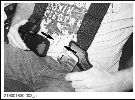
On both sides, adjust the seat belt tightly against your body by pulling the excess of the lap belt towards the inside. The buckle must be centered at the waistline (as low as possible).
