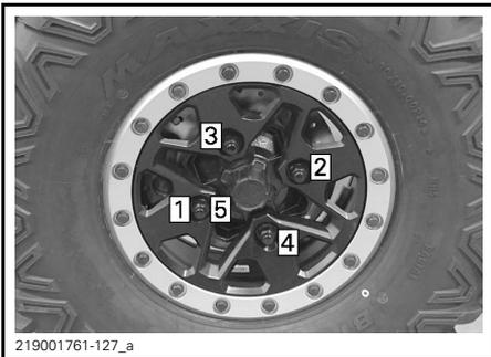
**NOTICE** Always use the recommended wheel nuts for the type of wheel. Using a different nut could cause damages to the rim or studs.
