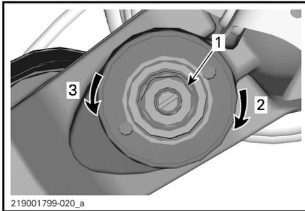
**HIGH SPEED COMPRESSION DAMPING (USE A 17 MM WRENCH)**
