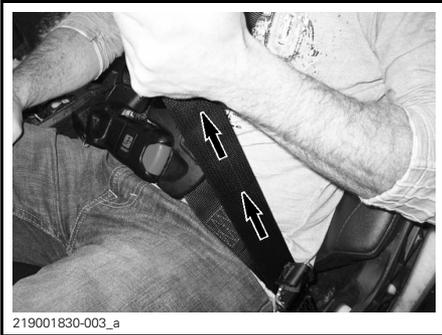
To loosen the seat belt, hold the lap belt with one hand and pull the red strap outwards.
