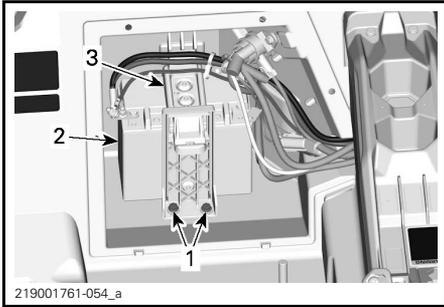
1. Battery holder retaining screws
