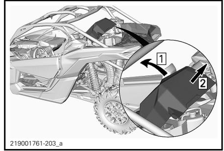
Remove CVT filter from vehicle.
