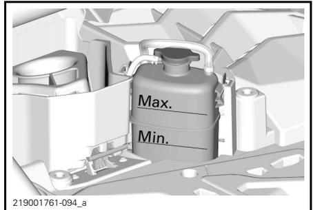
5. Add coolant in system as necessary. Use a funnel to avoid spillage. **Do not overfill.**
