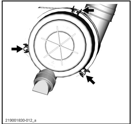
Remove the filter cartridge.
