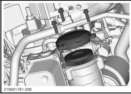
Install the cover on the engine.
