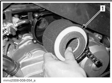
REMOVE AIR FILTER FROM HOUSING
