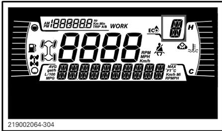
This display shows gear position of gearbox:
