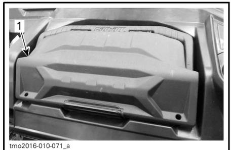
To open tool box, unlock panel and lift lid.
