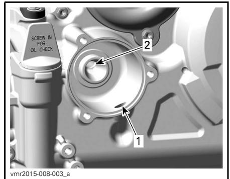
1. Inlet bore from the oil pump to the oil filter
