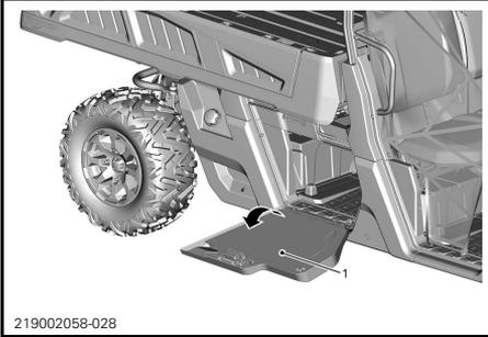
Remove battery cover by unscrewing the two 1/4 turn fasteners.
