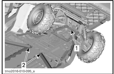
1. Lifting location under trailer hitch
