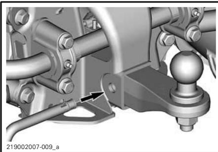
Secure the pin by folding the lock.
