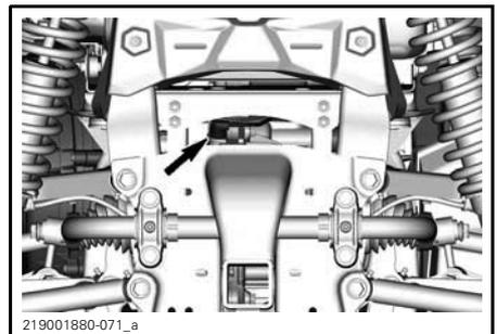
Under the vehicle, place a drain pan underneath the oil drain plug area.
