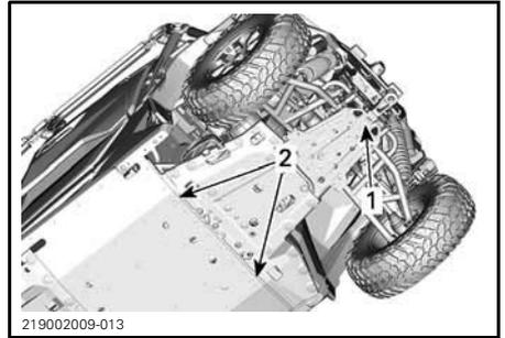
1. Lifting location under skid plate
