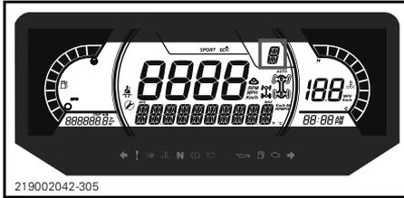
This display shows gears position of gearbox:
