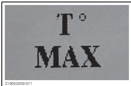
**NOTE:** In either T° MIN or T° MAX position, the system can not regulate a stable temperature.
