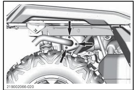
**TAIL PIPE RETAINING SCREWS**
