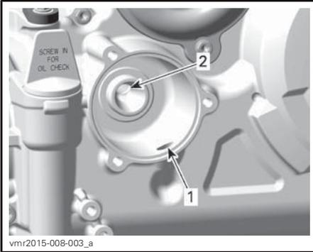
1. Inlet bore from the oil pump to the oil filter
