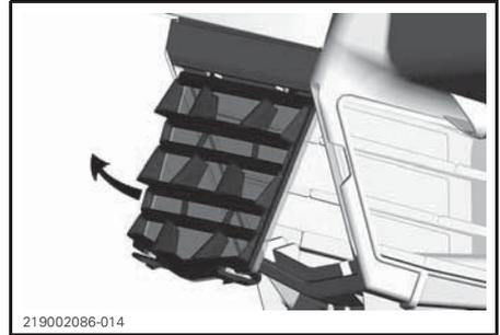
Clean air filter by washing it in lukewarm water with mild soap. Remove excess water and air dry before installation.
