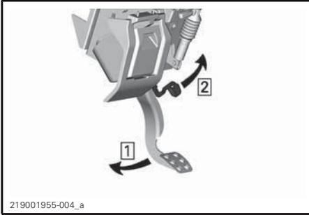
Step 1: Apply and hold brake pedal
