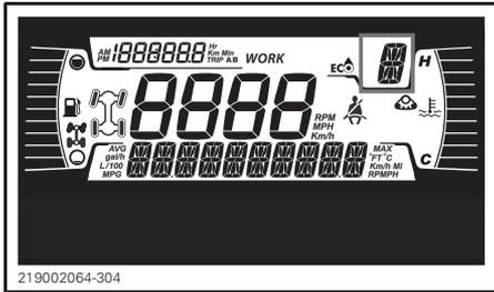
This display shows gear position of gearbox:
