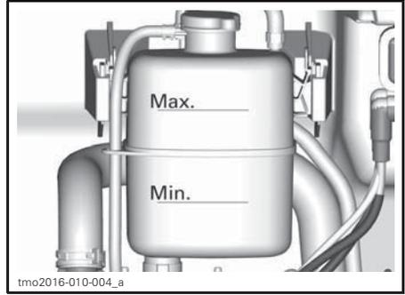
5. Add coolant in system as necessary. Use a funnel to avoid spillage. Do not overfill.
