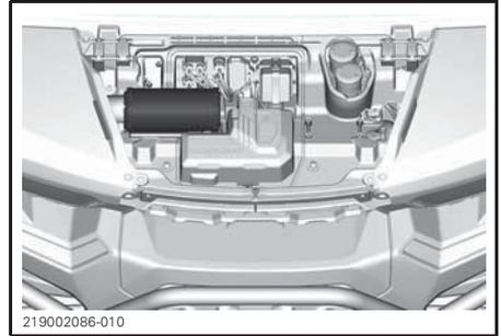
Lift and slide filter to remove.
