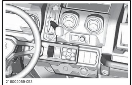
This switch selects 2 wheel drive or 4 wheel drive mode when the vehicle is stopped and the engine is running.
