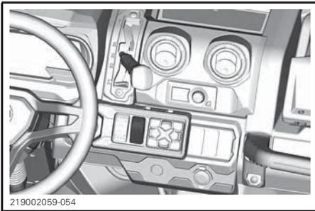
The differential switch enables locking of rear differential.
