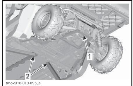
1. Lifting location under trailer hitch
